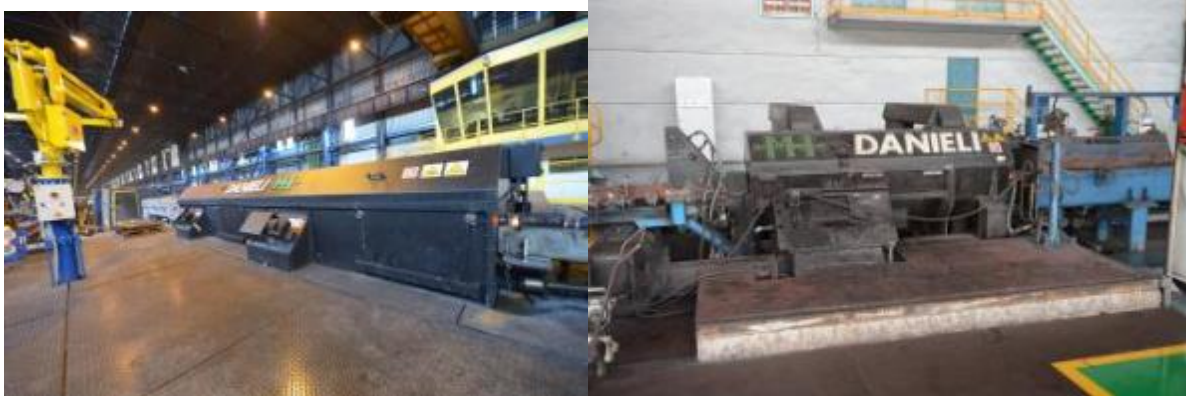
Figure 3. 4-stand and 2-stand PFB Blocks in operation at Ferriere Nord Italy and Angang Anshan I&S P.R. Of China.
