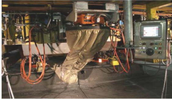
Figure 7. Danieli robotics utilization shown herein for mold powder application. Other applications include tundish temperature sampling and SEN exchange.
