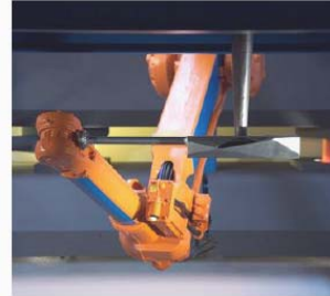
Figure 7. Danieli robotics utilization shown herein for mold powder application. Other applications include tundish temperature sampling and SEN exchange.
