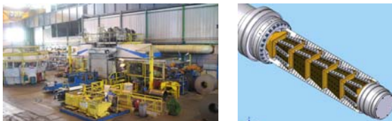
Figure 10: Reversing Cold Mill in St Chely and applied pyramidal type mandrel
