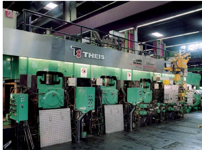
Figure 8: 4-stand tandem mill with changeable CVC ® plus 4-high / CVC ® plus 18-high insert in stands 3 and 4.
