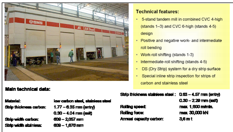
Figure 10: Main technical data and features of the CTCM at AK Steel.
