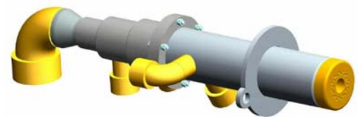
Figure 3. Oxygen Jet + Burner, with shrouding effect
