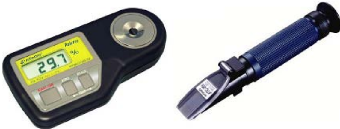
Figure 2. Typical Refractometer used to verify polymer quenchant concentration.
