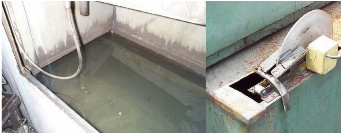
Figure 3. Dirty quench tanks and poorly maintained skimmers contribute to non-uniform quenching and are sources of nutrients for biological growth.
