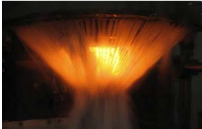
Figure 6. Non-uniform quenching due to plugged nozzles.
