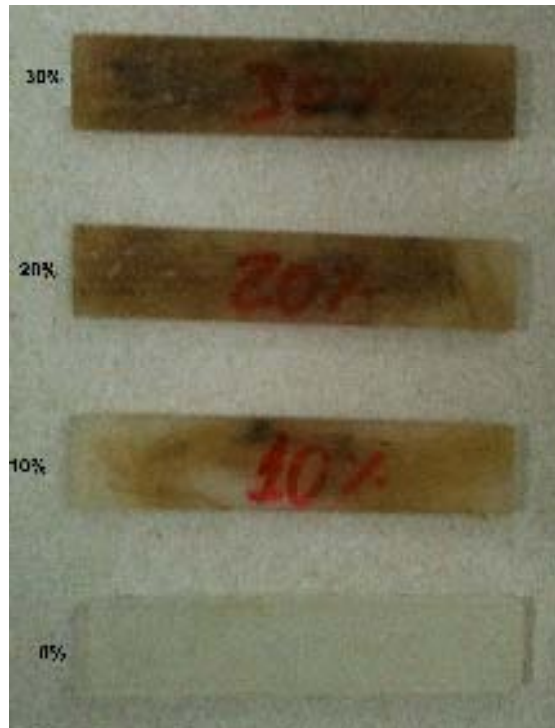
Figure 3. DMA specimens of DGEBA/TETA epoxy composites incorporated with different volume fractions of ramie fibers
