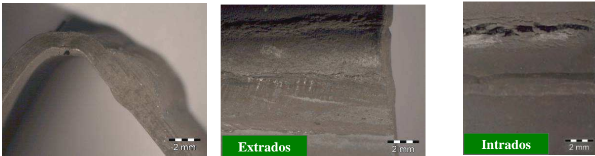
Figure 12 : Binocular examination - K44X/430LNb.
