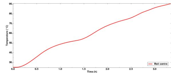
Figure 4: the evolution of the work-roll temperature at its centre.
