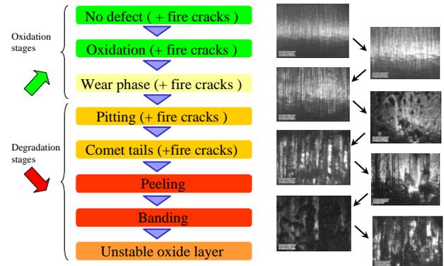
Figure 1: work-roll degradation process, with two subsequent phases: the oxidation stages then the degradation ones.
