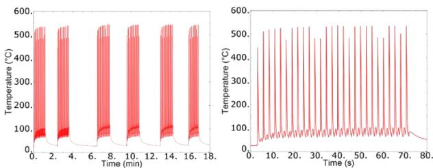
Figure 6: [Left] work-roll surface temperature evolution for the first six strips of the rolling campaign; [Right]: Focus on the first strip
