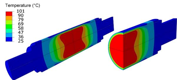
Figure 3: thermal field of the work-roll observed at the end of a rolling campaign.
