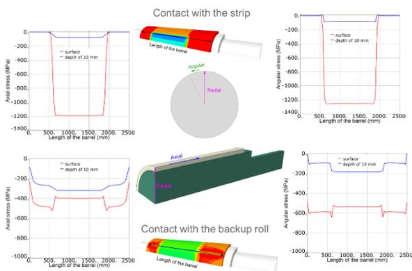
Figure 8: axial (left) and angular (right) stresses variation along the roll barrel length
