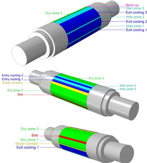
Figure 2: the thermal boundary conditions applied to the work-roll.
