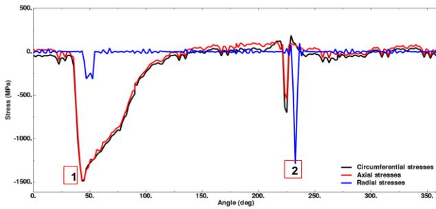
Figure 7 : comparison between the radial, axial and circumferential stresses of the roll. (1) the contact angle between the strip and the work-roll is fixed to 8 degrees and 2 degrees between the work-roll and the backup roll (2)
