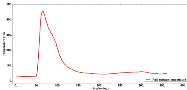
Figure 5: fast thermal evolution of the work-roll
