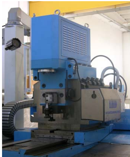
Figure 8: Turning and Notching group
