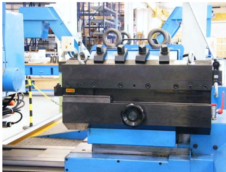
Figure 6: Atomat's tool saddle group
