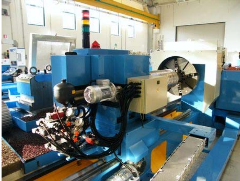
Figure 7: Quill and tailstock motorization
