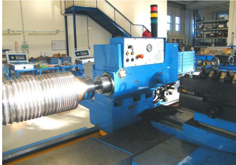
Figure 5: Atomat's tailstock assembly
