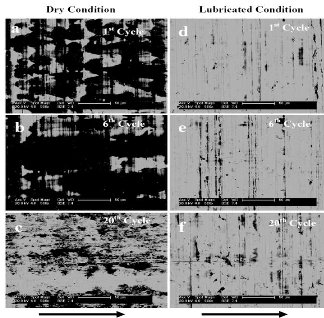
**Figure 5:** Backscattered SEM of steel plates when Al-4Mg alloy pin slid on steel plates at 1<sup>st</sup> (a, d), 6<sup>th</sup> (b, e) and 20<sup>th</sup> (c, f) cycles under dry (a, b, c) and lubricated (d, e, f) conditions. Sliding direction is perpendicular to the unidirectional grinding marks. The arrows indicate the sliding direction of the pin relative to the plate.
