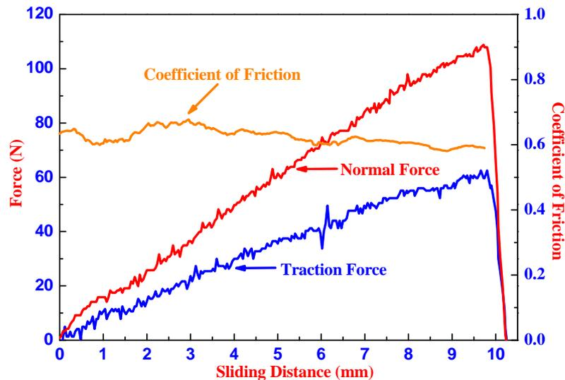
**Figure 1:** Variation of forces and coefficient of friction with sliding distance.
