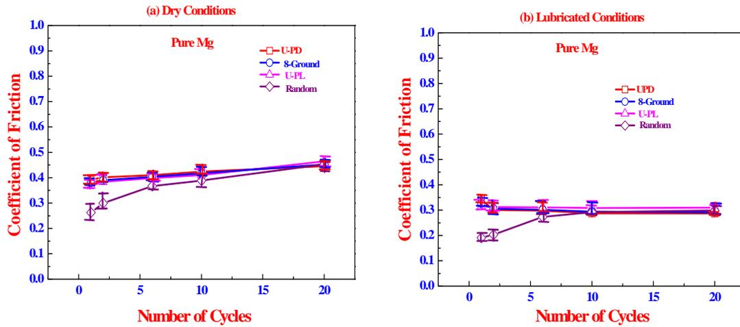
**Figure 4:** Variation of average coefficient of friction with number of cycles when pure Mg pin slid on steel plate of different surface textures under (a) dry and (b) lubricated conditions.
