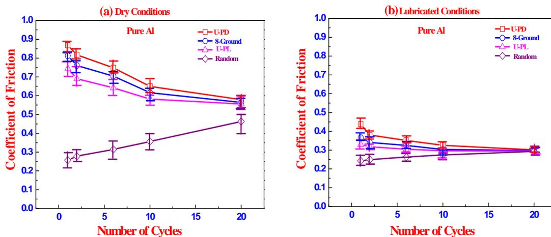
**Figure 3:** Variation of average coefficient of friction with number of cycles when pure Al pin slid on steel plate of different surface textures under (a) dry and (b) lubricated conditions.
