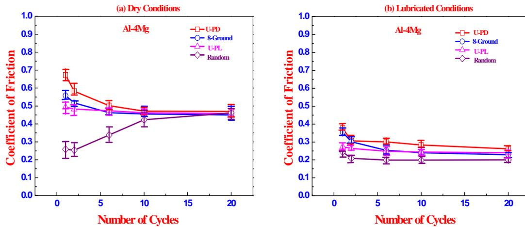
**Figure 2:** Variation of average coefficient of friction with number of cycles when Al-4Mg alloy pin slid on steel plate of different surface textures under (a) dry and (b) lubricated conditions.
