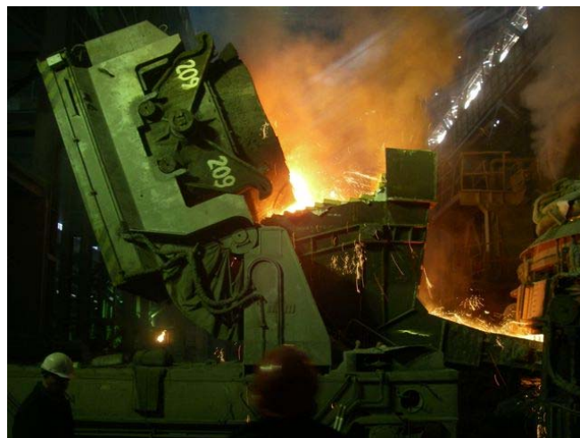
Figure 8: Picture of Hot Metal Charge with door launder
