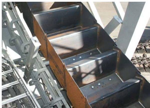
Figure 12: Conveyor system for Hot DRI
