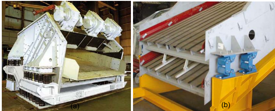
Figure 9. (a) Two stage helical spring isolator; (b) Rosta isolators. (10,11)
