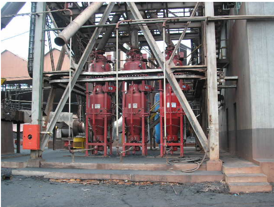
Picture 02: charcoal pneumatic injectors – Clyde Materials Handling
