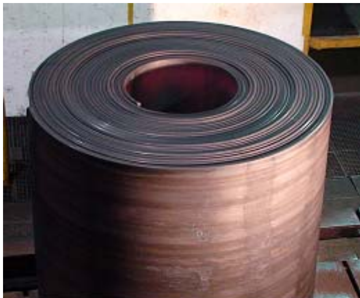
Figure 6: First X70 coil with a thickness of 25 mm.
