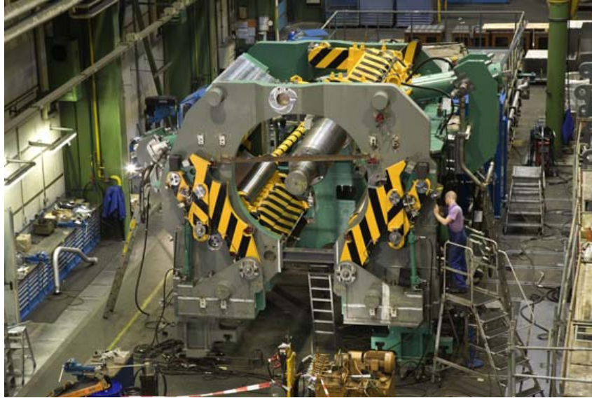
Figure 4: Preassembly and functional tests at SMS Siemag workshop.
