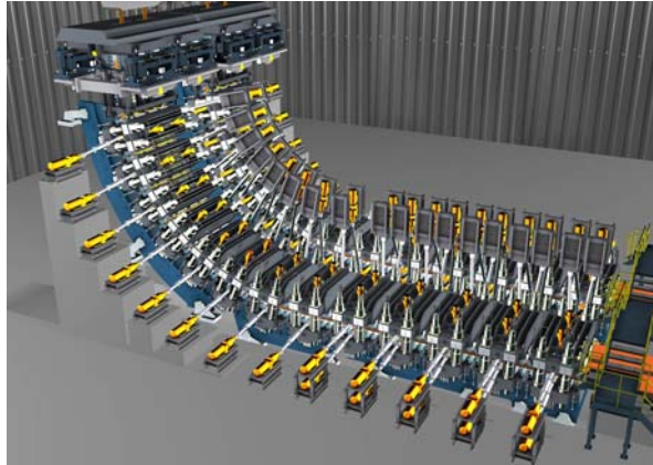
Figure 8. General View of the Strand Guide of a VAI Compact Caster (one line)
