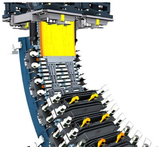
Figure 10. Dummy Bars for two Small Slabs Equipped with Wide Slab Head
