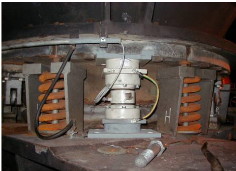
Old Concept – 1978 - Load cell / spring / tie rods and torsion links
