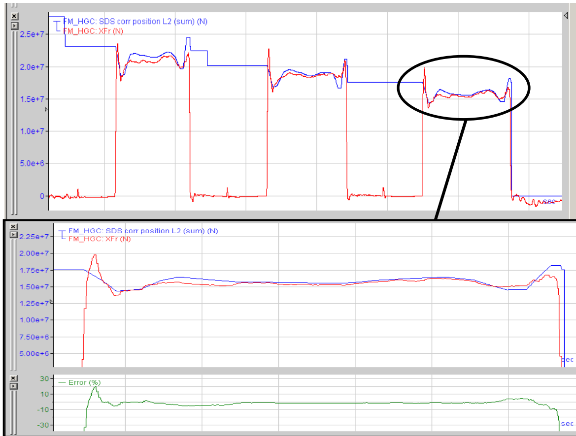
Figure 11. 20 point setup showing predicted (blue), measured (red) rolling load & error (green).
