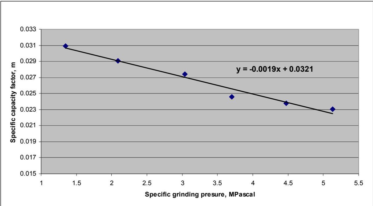
**Figure 1:** variation of the specific capacity factor with grinding pressure and calculated trend line.
