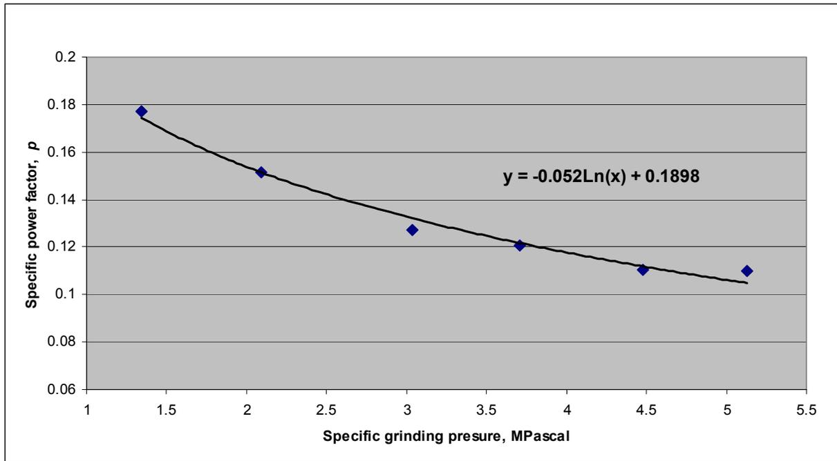
**Figure 2:** variation of the specific power factor with grinding pressure and calculated trend line.
