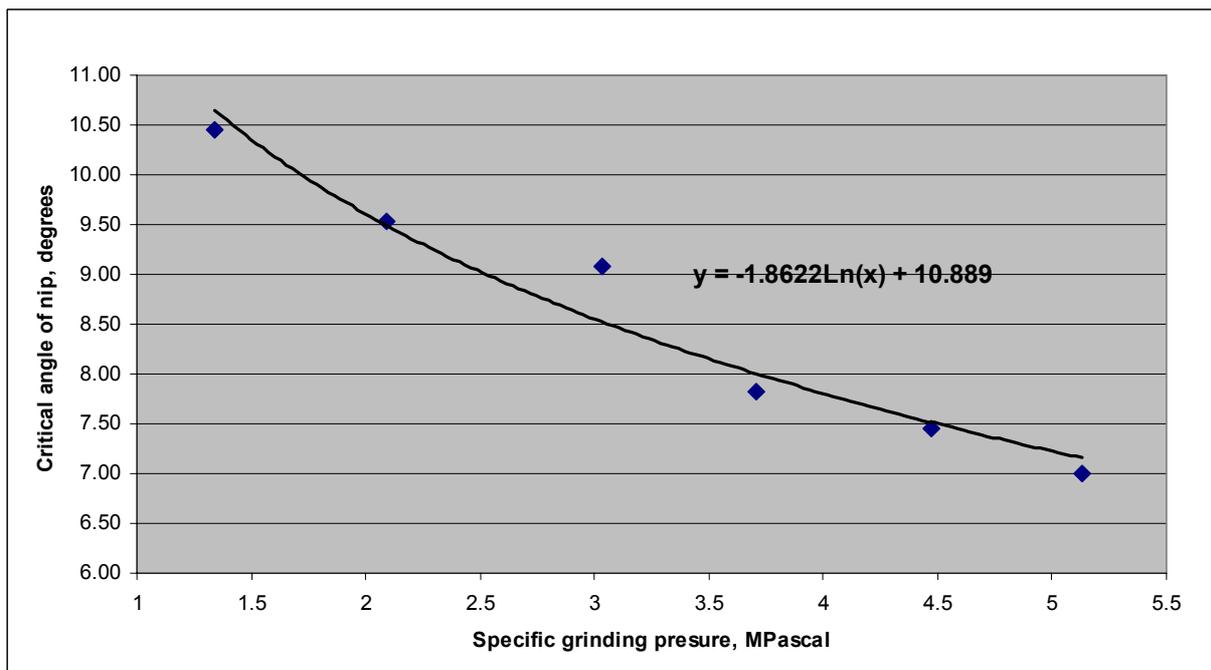
**Figure 3:** variation of the critical angle of nip with grinding pressure and calculated trend line.
