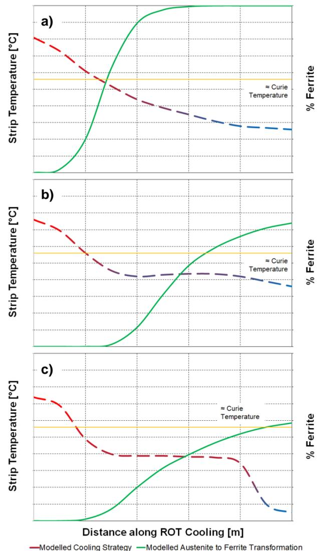
**Figure 4.** Comparison of cooling strategy and predicted transformation along the ROT cooling for 3 steel groups; a) conventional Low Carbon steels, b) conventional Structural steels and c) Advanced High Strength steel – Dual Phase (DP) steels.
