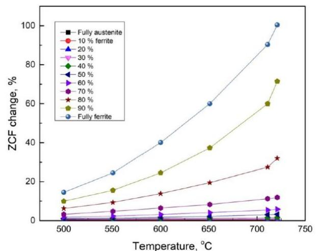
**Figure 3.** Predicted ZCF values for ferrite-austenite microstructures (0-100% ferrite) against temperature [8].
