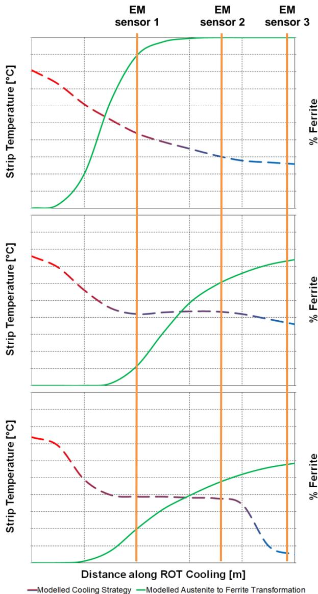
**Figure 5.** An update of Figure 4 with an example of 3 locations for 3 Transformation Monitor EM Sensors in the ROT.
