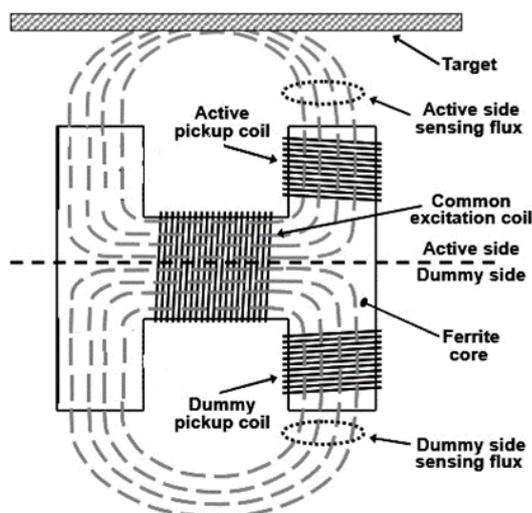
**Figure 2.** A schematic diagram of an H shaped sensor such as the type used in the EMspec<sup>TM</sup>. [8]
