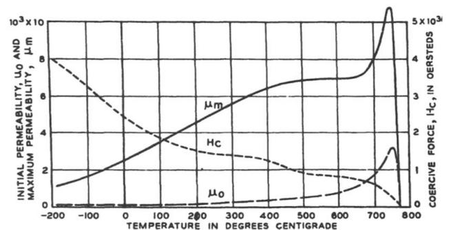
Figure 1. Temperature dependency of initial magnetic permeability  $\mu_0$  for iron [2].
