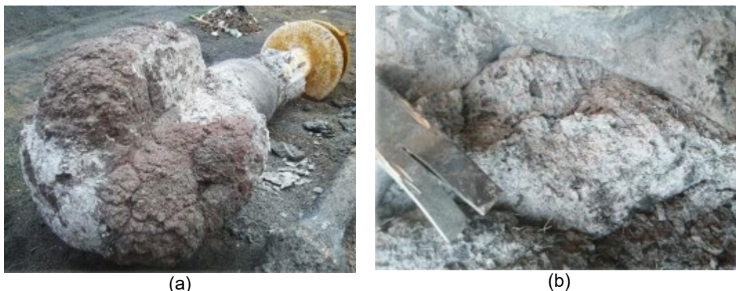
Figura 11. Post-mortem: (a) Impeller KR after 430 heats and (b) recycled aggregates of \text{Al}_2\text{O}_3\text{-SiC} preserved on refractory concrete.
