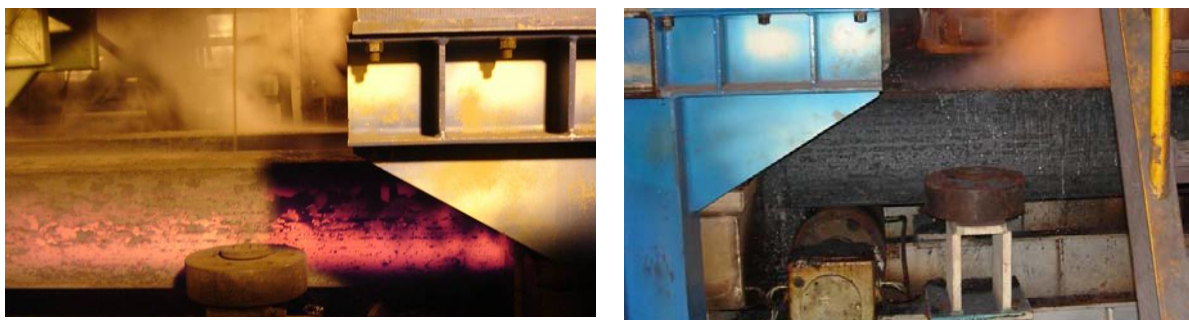
Figure 6. visual effect when using Quench box; bloom surface became completely black after.
