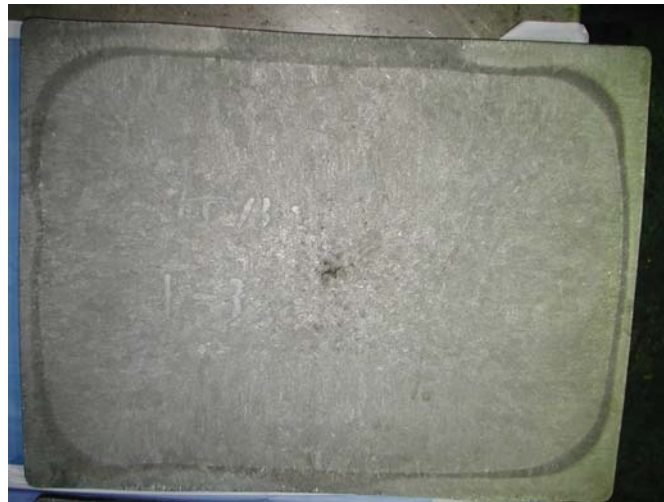
Figure 8. transversal section on KSG4120H – low carbon Niobium steel grade, casting speed 0.61 m/min , Quench box water flow 1100 L/min. It is evident the effect of quenching on the entire perimeter with a quenched deep 15-20 mm.
