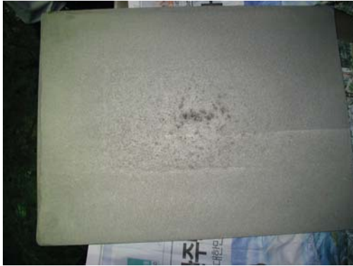
Figure 2. STB 2 bearing steel 0.52 m/min, tundish SH +30°C, height reduction 7 mm applied with 5 rolls.
