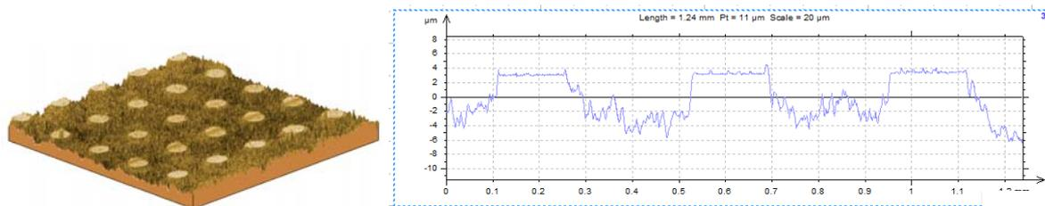
**Figure 4.** Example of the surface topography of a textured samples containing pillars using a negative photoresist; left, perspective view; right, line profile.
