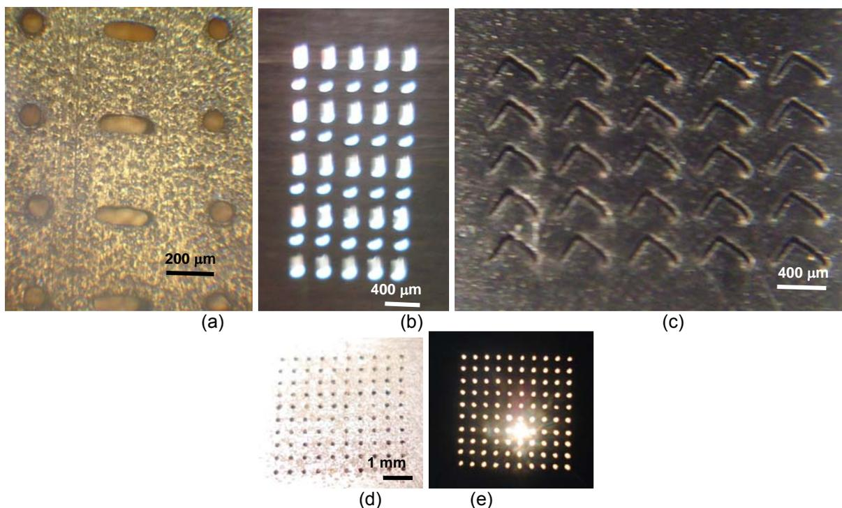
**Figure 8.** Examples of the use of EDM to machine the tool covers: (a) EDM tool with array of dashed lines and dots which produced the tool cover in (b); (c) tool cover produced by EDM with array of chevrons; (d) tool cover with array of dots before painting; and (e) after painting.
