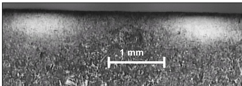
**Figure 11.** Optical micrograph of the cross-section of two hard martensitic stripes (white etching) produced in a low-carbon steel sample.
