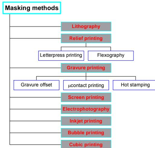
Figure 2. Schematics of the tree structure for methods for mask generation.
