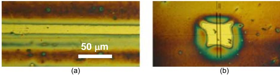
**Figure 7.** (a) 20 μm gap between parallel printed lines; (b) 40 μm square gap.
