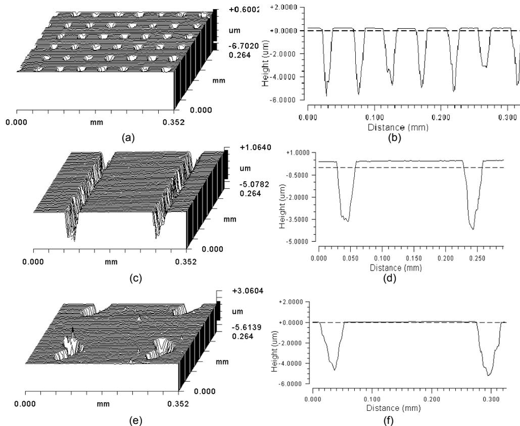
**Figure 3.** Examples of the surface topography of textured samples using a positive photoresist; left, perspective views; right, line profiles.
