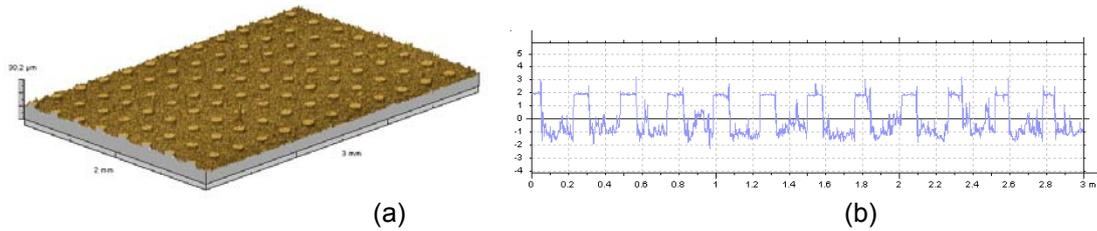
**Figure 6.** Surface topography sample printed with dots after etching and stripping; (a). 3D map; (b) line profile.
