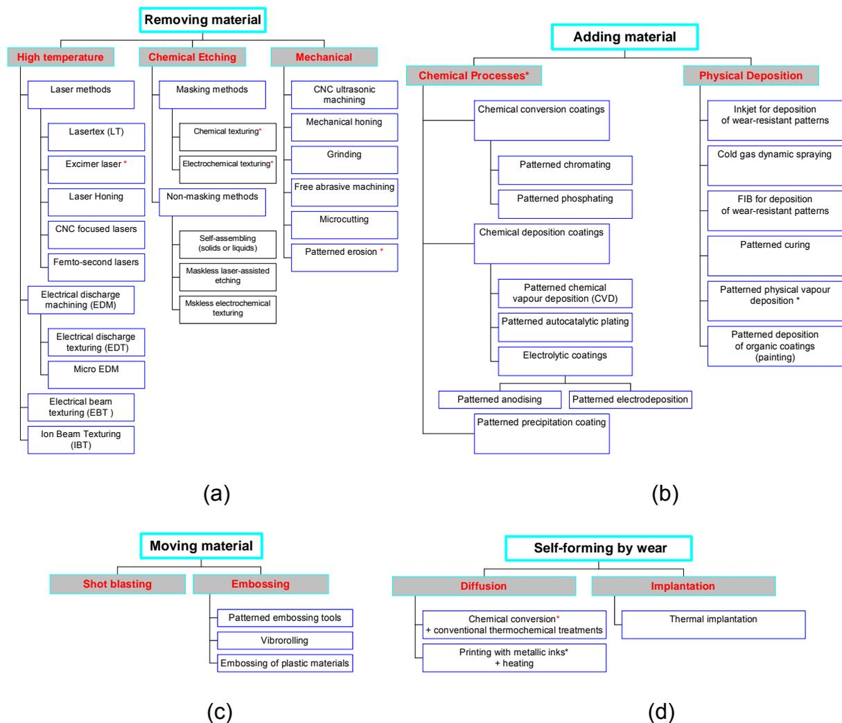
**Figure 1.** Schematic representation of the tree structures for methods involving: (a) removing material; (b) adding material; (c); moving material; (d). self-forming by wear.
