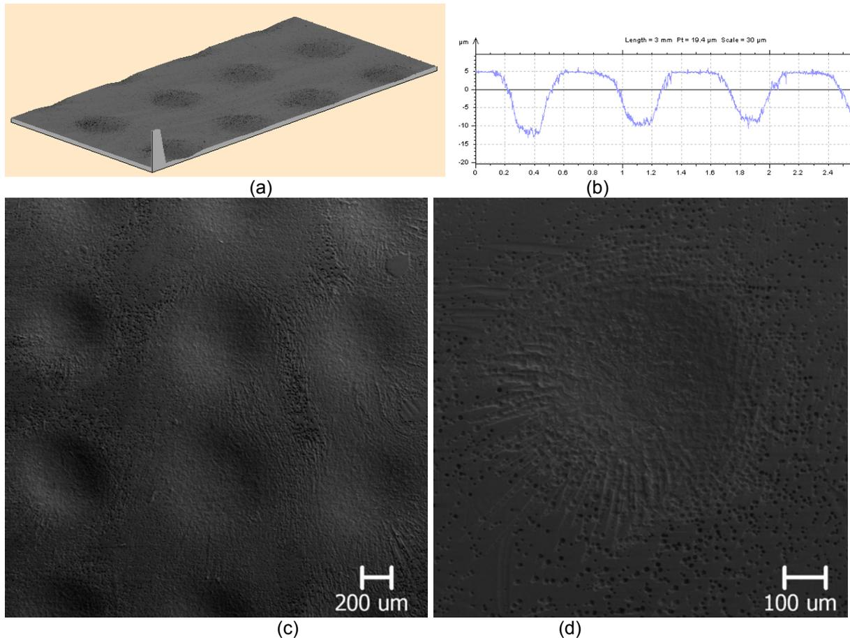
**Figure 9.** Example of a steel sample textured by MECT; (a) interferometric map; (b) profile across a line of circular pockets; (c) and (d) SEM images.
