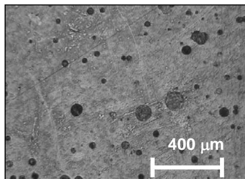
**Figure 10.** Textured steel surface obtained by mixing 50 ml of olive oil, 4 g of stearic acid and 25 ml of nitric acid solution (10%), etching time = 3 min.
