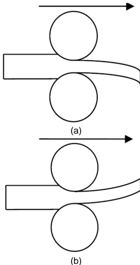
**Figure 1.** Curvature at the tip of the strip: (a) "turn-down"; (b) "turn-up".
