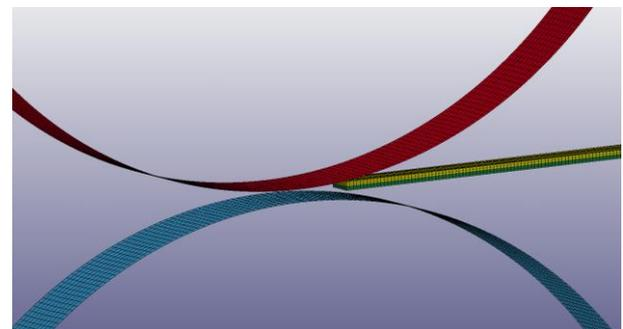
**Figure 4.** Typical finite element mesh used in the models.
