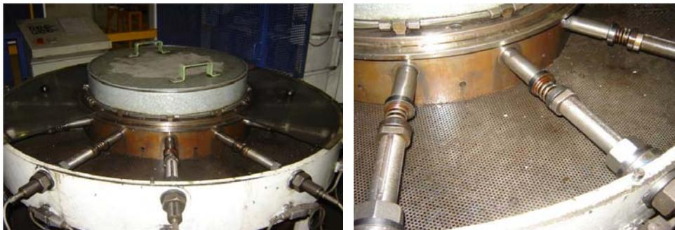
**Figure 12.** Bench used for the experimental fatigue test showing samples during cyclic loading.
