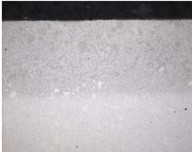
Figure 2. No occurrence of carbide precipitation in innovative nitriding.
