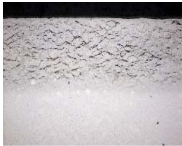
Figure 1. Typical GNS layer showing fine carbides precipitated at grain boundaries.
