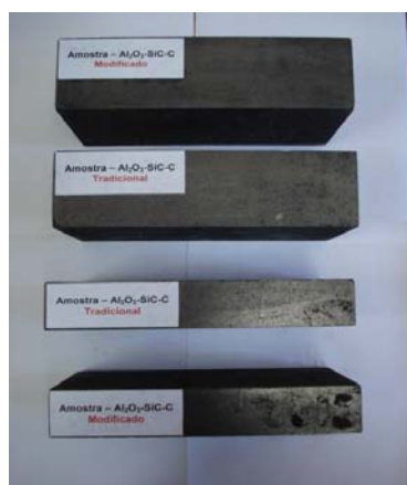
Figure 6- Sample preparation for laboratory tests.
