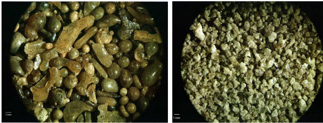
Figure 7. Dry granulated slag/ Wet granulated slag.
