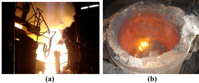
Figure 1 – Photo showing the added material during the tapping (a) and in the bottom of the ladle (b)
