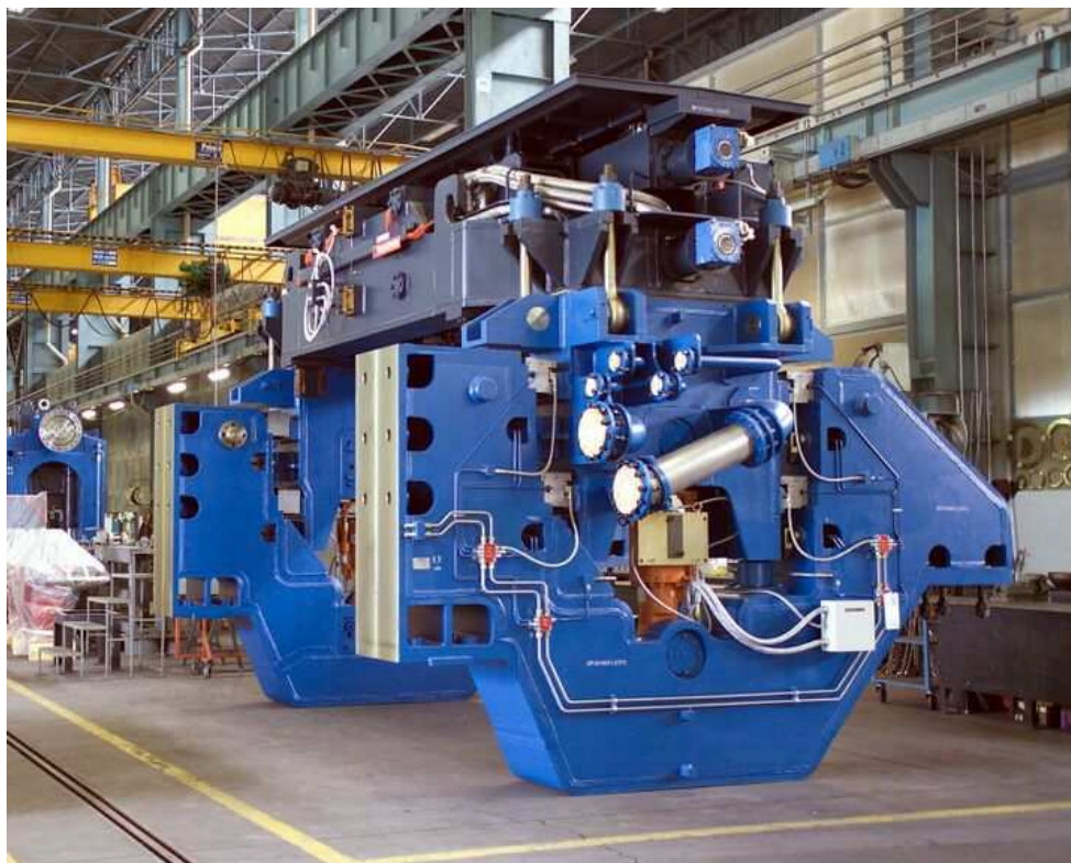
Figure 1 : INMO mould and oscillation system in operation in ArcelorMittal Dunkerque ( france) revamped casters
