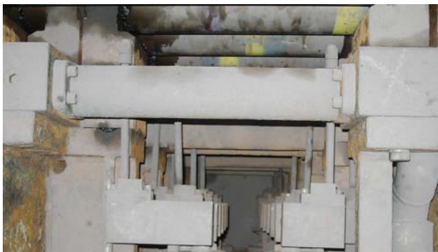
Figures 9 – “Inline” nozzle layout causing temperature striping.
