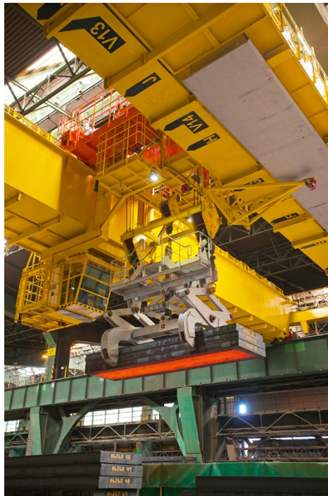
Figure 3. The “automatic crane package” at ArcelorMittalDunkerque, France, recognizes the real position of the slabs to be picked up, and also to positively identify each slab for tracking purposes.
