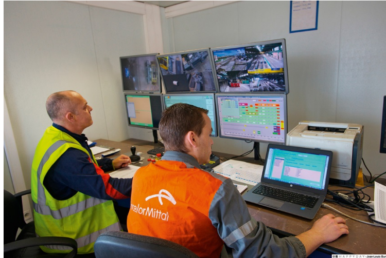
Figure 2. Remote pulpit room of the Automatic Crane for slab yard at ArcelorMittalDunkerque, France.
