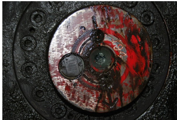
Figure 7. RFID Tag mounted on roll neck.
