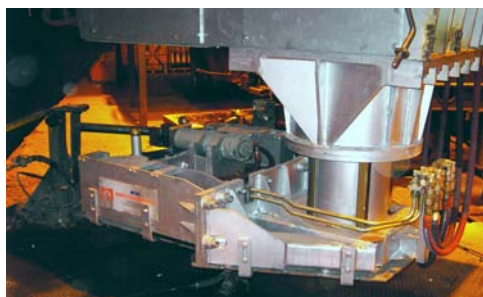
Figure 2: First fully automatic coupling of the casting cylinder.
