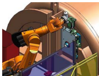
Figure 9: Coupling of mounting cylinder with SNAP coupling.
