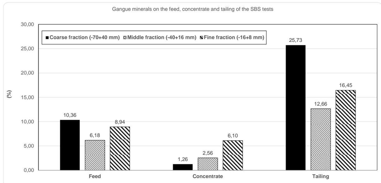
Figure 6: Gangue minerals in the feed, concentrate and tailings after testing
