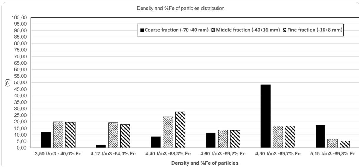
Figure 5: Distribution of density and %Fe of particles
