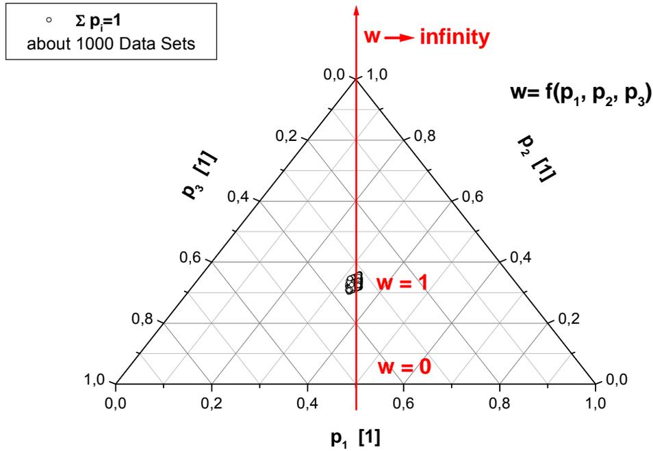
**Figure 4.** Selection of 1000 central range points of the ternary non-dimensional meniscus parameter diagram including slab and thin slab data.
