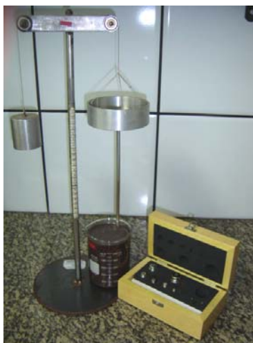
Figure 1. Counter-balance system for the penetration test.
