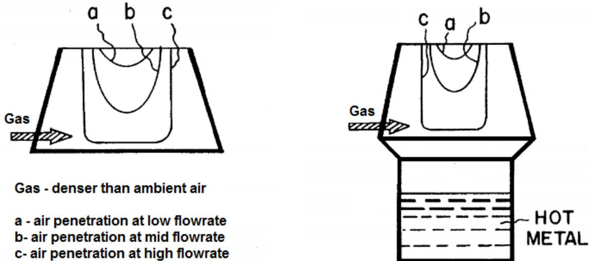
Figure 2. Air penetration profile for swirling flow at different inert gas flowrates. [5]
