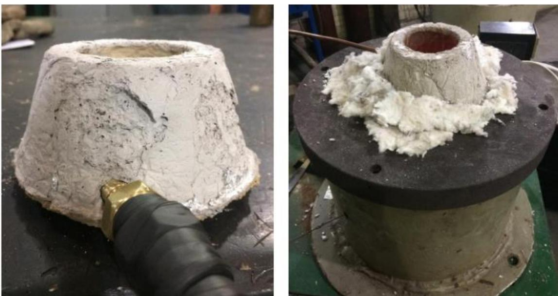
**Figure 4.** Refractory cone and apparatus assembled.
