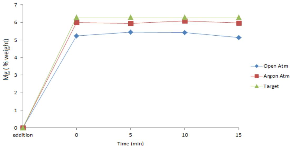
**Figure 5.** Magnesium content in the different castings in function of time.
