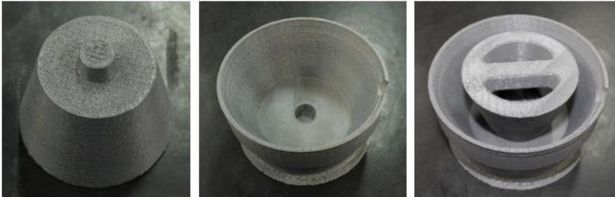
**Figure 3.** 3D-printed ABS-die.
