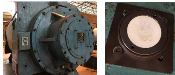
Figure 5. Sensor installed on chock
