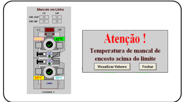
Figure 8. Alert Indication on HMI
