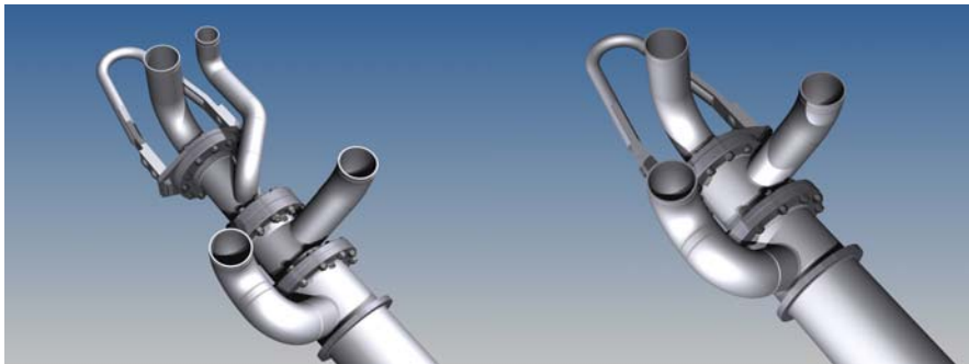
Figure 3. Split flow post combustion top adaptor on the left; double flow post combustion top adaptor on the right
