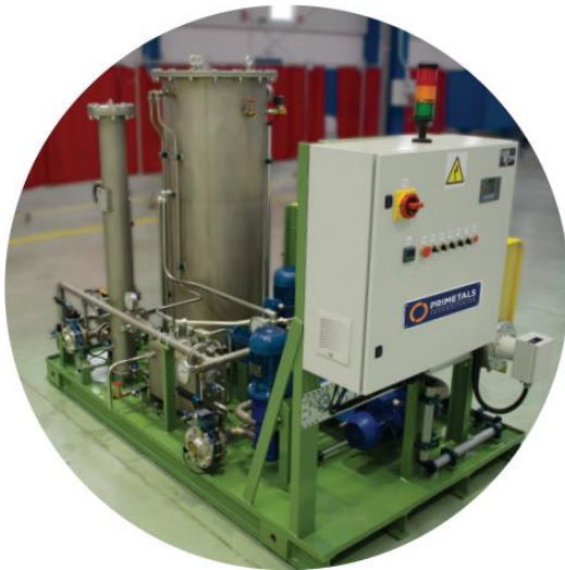
Fig. 13 – Vacuum Dehydration System
