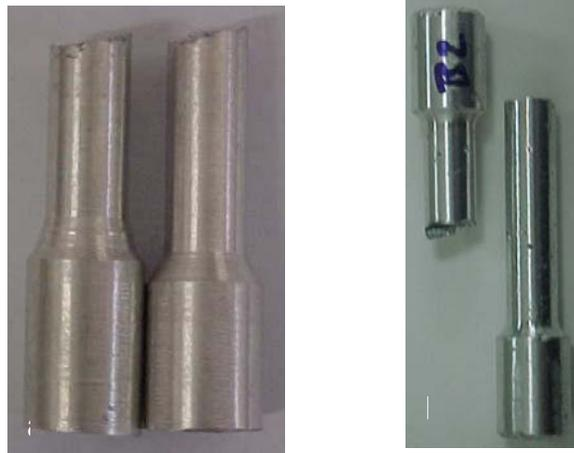
**Figure 5** – Shape of fracture surface the specimens. a) sample by mold with copper b) sample by mold with steel.
