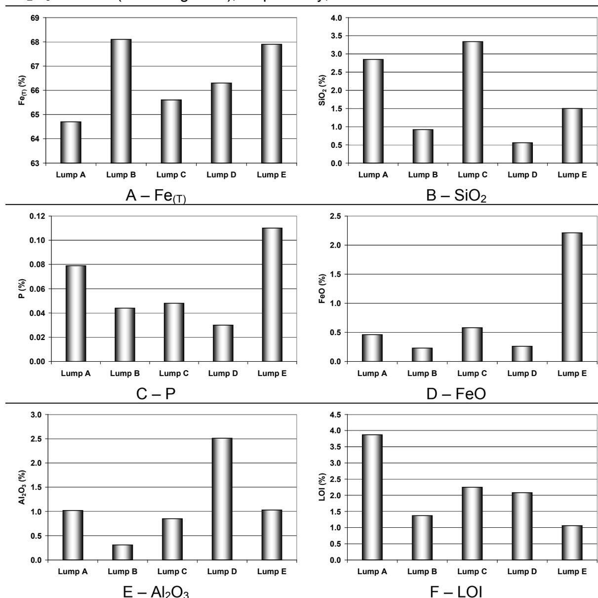
**Figure 2.** Results of chemical analysis of lump ores used in Usiminas.
