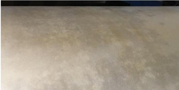
Figure 15: Barrel surface with “cloud-pattern”
