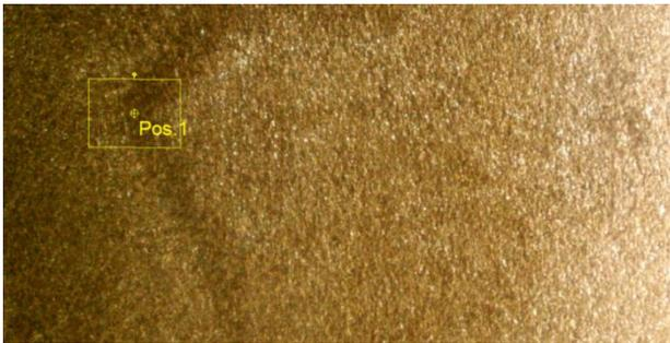
Figure 11: Detail of degenerated carbides in Figure 10
