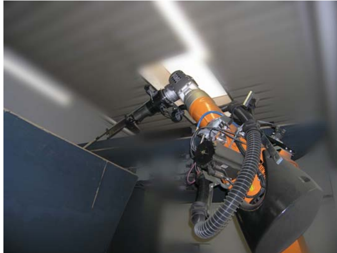
Figure 10. Sampling from tundish
