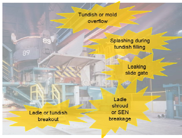
Figure 1 Dangers on casting platform
