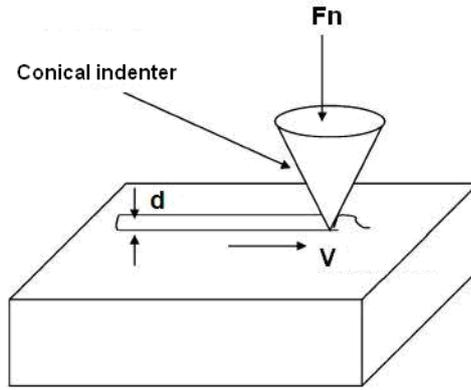
**Figure 4** – Illustration of a scratch test.  $F_n$  is the normal load,  $d$  is the size of the groove and  $V$  is the velocity of the translation motion.<sup>[21]</sup>
