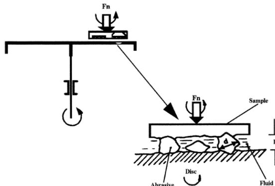
**Figure 2** – Illustration of LTM test.<sup>[13]</sup> Fn is the normal force.
