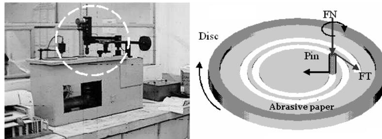
**Figure 3** – Illustration of pin-on-disk test.<sup>[18]</sup>
