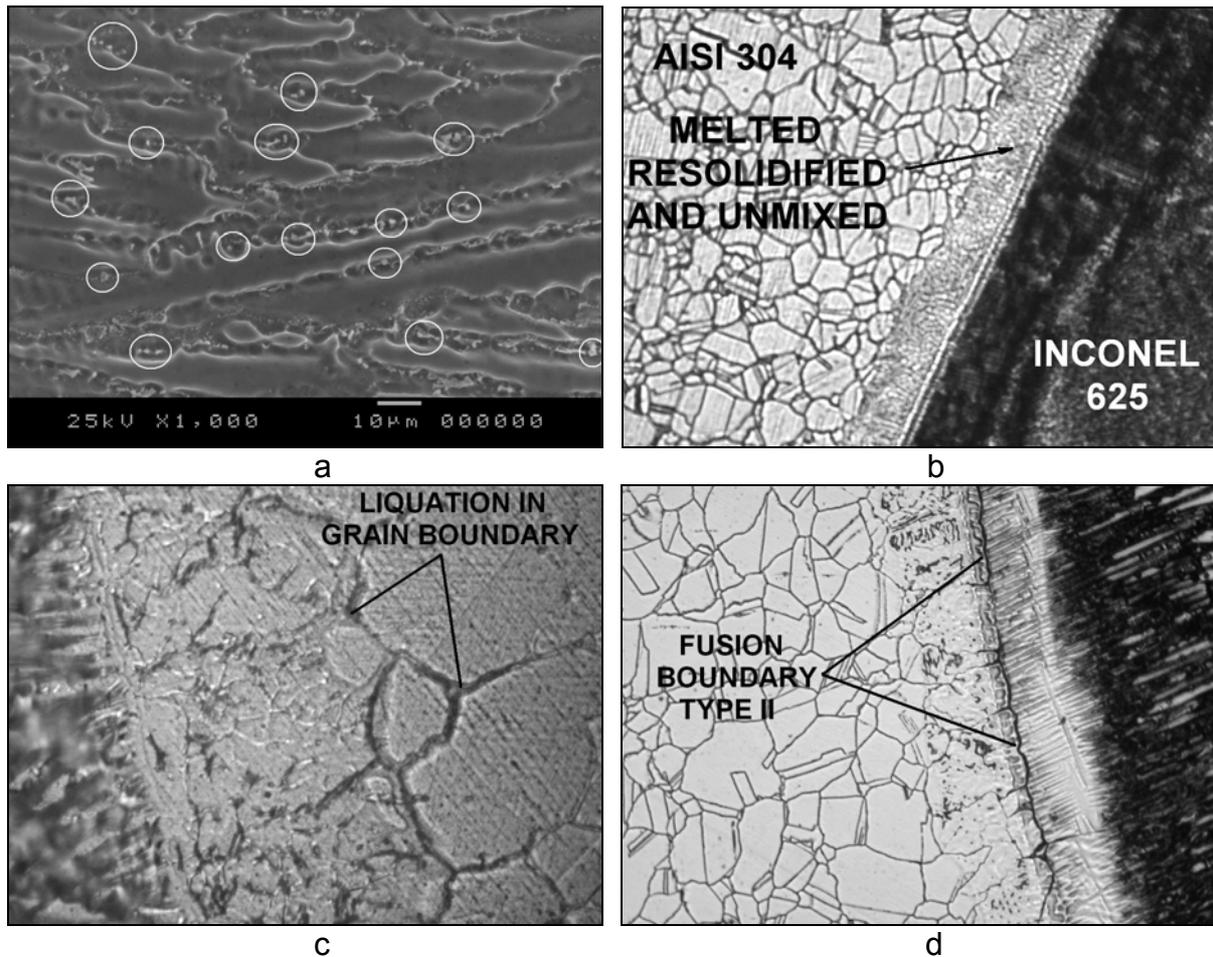
**Figure 4.** Micrography of the weld joint. Precipitation in dendrite boundary, circle in weld metal (a), melted and unmixed zone in HAZ (b), HAZ liquation in grain boundary near the fusion line as welded (c), fusion boundary Type II sample after PWHT (800°C for 3 h) in fusion line (d).
