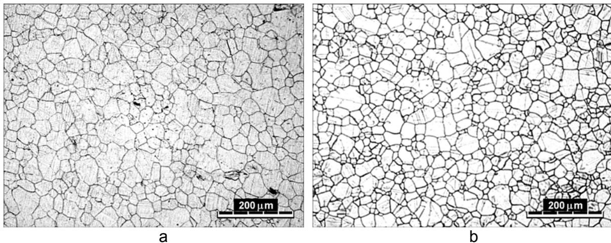
**Figure 1.** Micrography of the AISI 304, austenitic grain (a) as supplied and (b) after heat treatment (800°C for 3 h), with some coarse grain boundary. The grain size of the AISI 304 did not change appreciably after the heat treatment.
