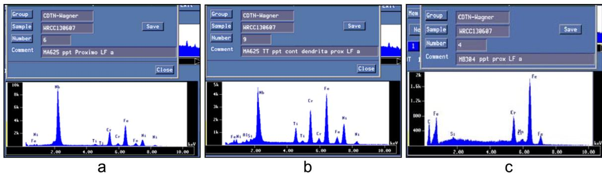
**Figure 5.** EDS spectra in the weld metal Inconel 625 Niobium precipitate (a) in sample without PWHT and the Niobium, Titanium and Chromium precipitate in dendrite boundary (b) in sample with PWHT
