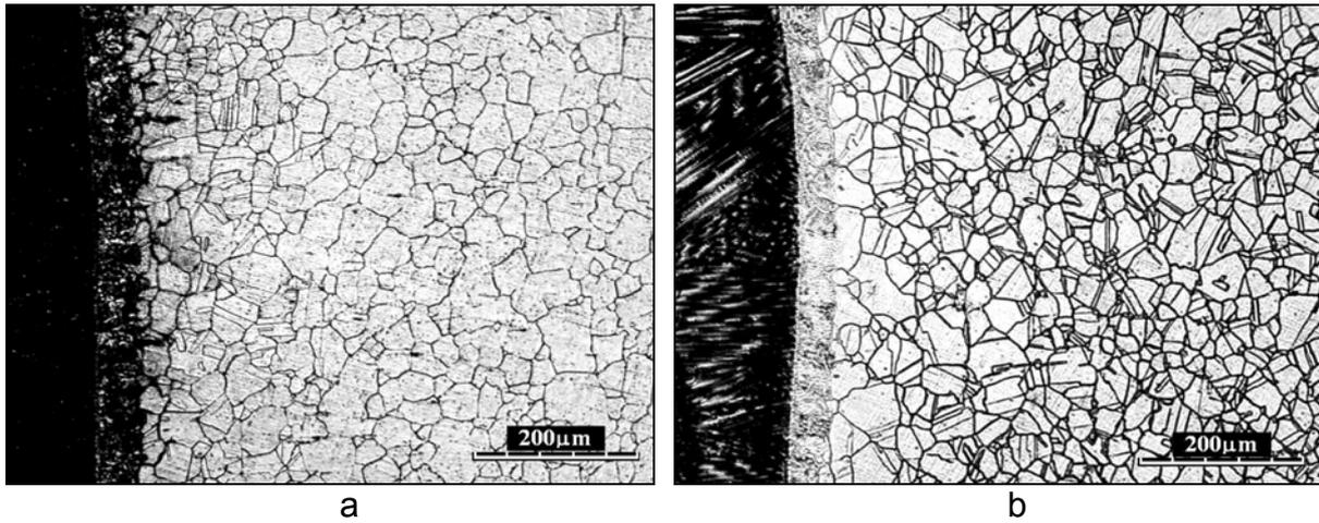
**Figure 2.** HAZ micrography. The sensitization in grain boundary near the fusion line, as welded (a) was lower with PWHT (800°C for 3 h) (b).
