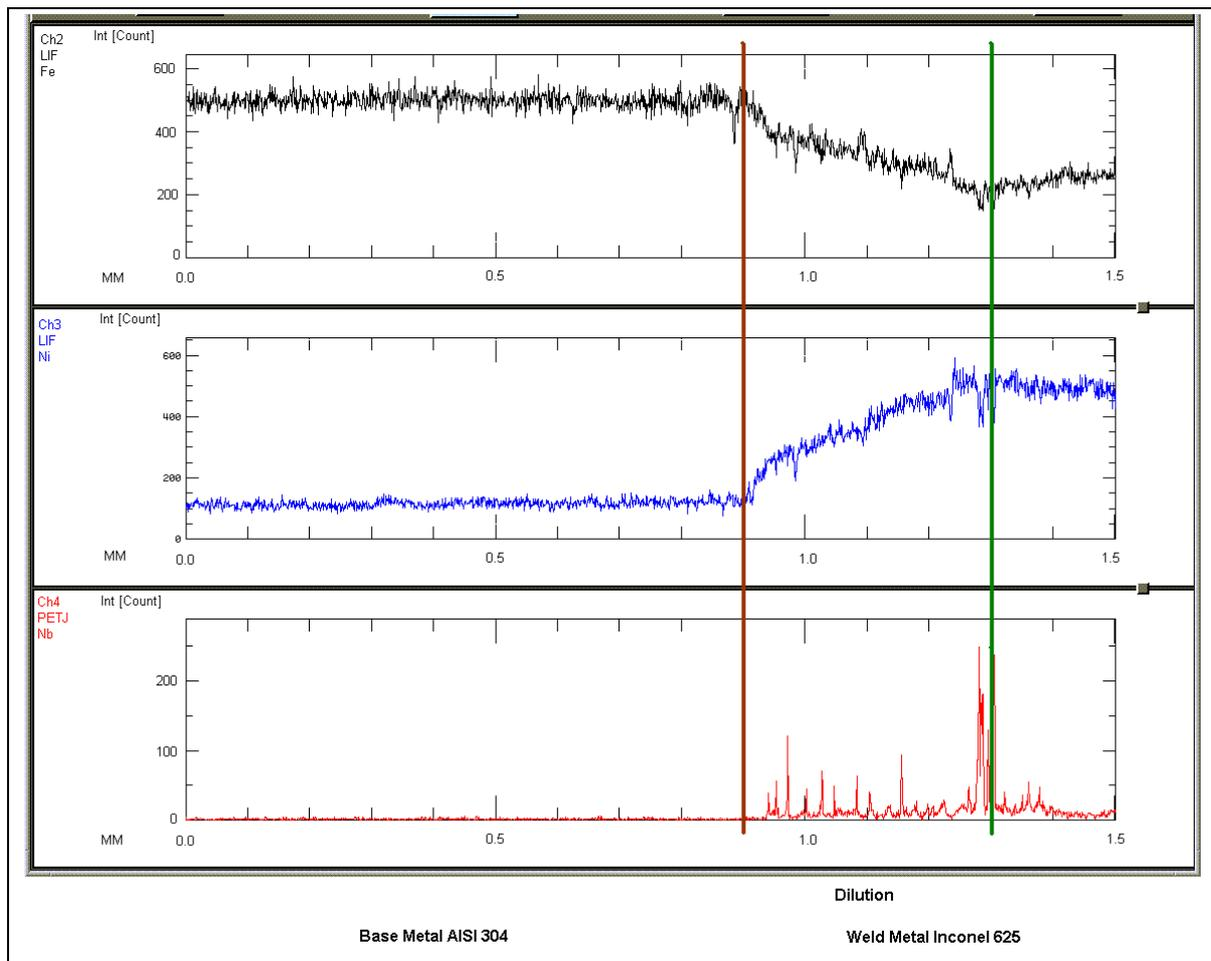
**Figure 6.** Composition profile of the Fe, Ni and Nb in dilution region of the BM AISI 304 in weld metal Inconel 625, without PWHT.
