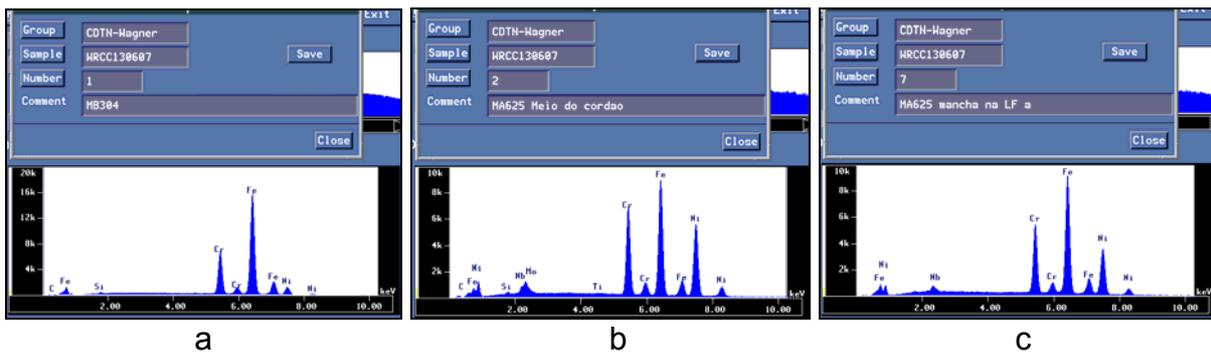
**Figure 3.** EDS spectra of the base metal AISI 304 (a), the center of the weld metal Inconel 625 (b), and dilution of the AISI 304 in Inconel 625 (c).
