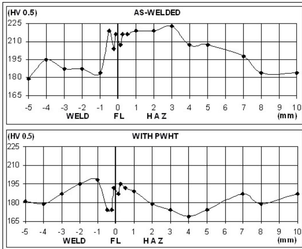
**Figure 7.** Cross-weld Vickers microhardness surveys of the samples. (a) as welded and (b) with PWHT (800°C for 3 h).
