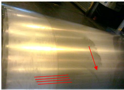
Figure 3. Backup roll of stand3 with chatter marks.
