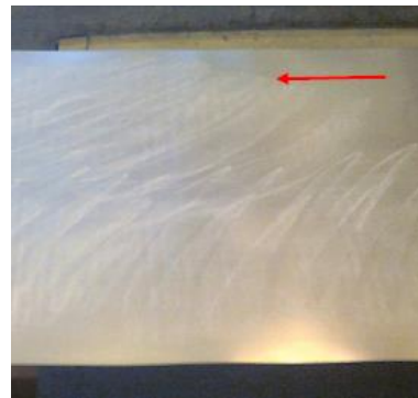
Figure 1. Fifth-octave chatter marks on steel strip.
