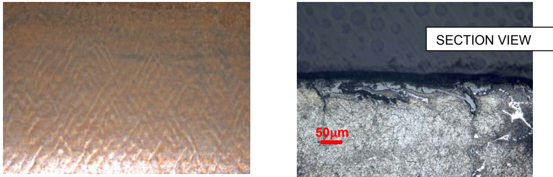
Figure 10 Surface of SemiHSS after a long campaign in R4 (340.000 ton)
