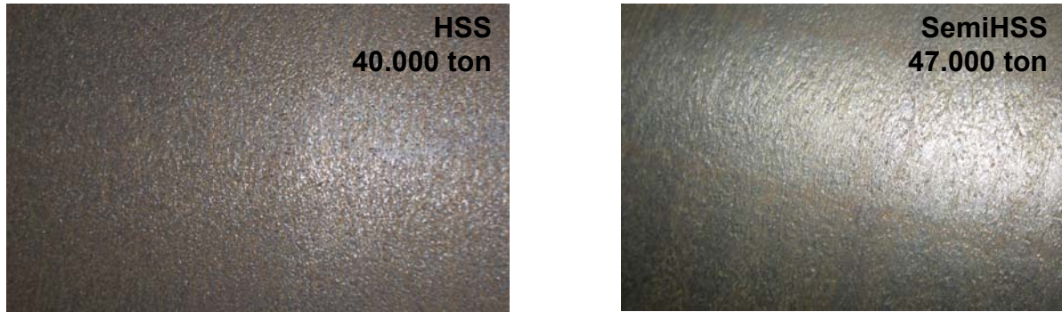
Figure 13 Aspect of the surface after a campaign in the reversing roughing stands
