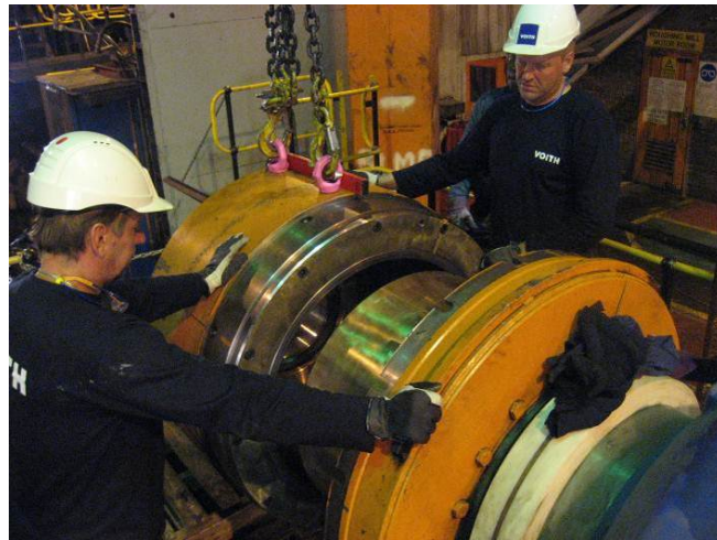
Figure 1. Disassembly of the Safeset from the motor shaft.
